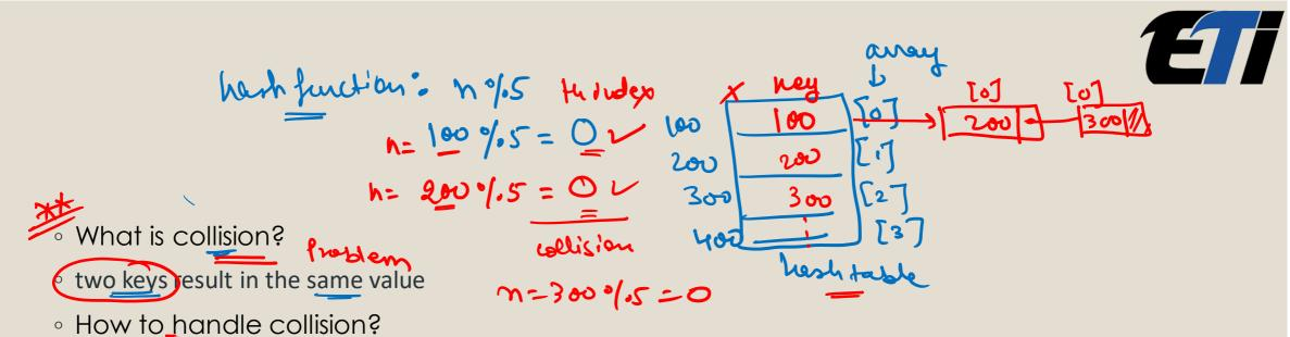
**Chaining: The** idea is to make each cell of hash table point to a linked list of records that have same hash function value. Chaining is simple, but requires additional memory outside the table.
